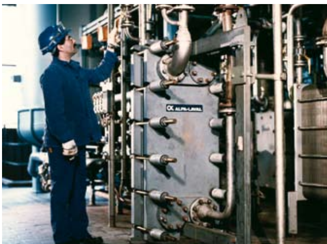
Alfa Laval DIABON® plate heat exchanger in F100 material used for cooling hydrochloric acid in a German plant.
