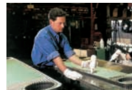
6. Regasketing. Selection of genuine spare parts to ensure optimal sealing performance, to increase uptime and to decrease operating costs. Alfa Laval helps determine the right gasket for your plate heat exchanger, based on media type, pressure and temperature.
