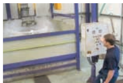
2. Gasket removal. Immersion of plates in liquid nitrogen at -196°C to make the gaskets brittle, causing them to shrink and to separate cleanly from the plate.
