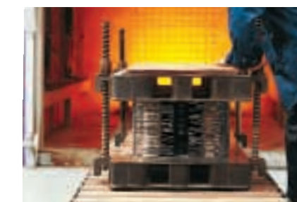
7. Oven-curing. Bonding of genuine gaskets to the plates using a unique, extra-strength Alfa Laval epoxy adhesive.
