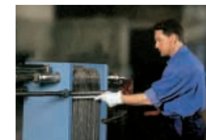
8. Pressure testing. As an option, Alfa Laval can verify the restoration of a leakage-free sealing function for the entire plate heat exchanger by pressure testing.
