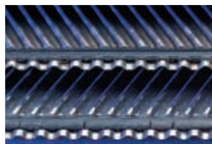
1. Plate inspection. Assessment of plate condition, upon arrival at the service centre, which includes thorough examination of all plates for any major deformations. This inspection ensures the plate can be reconditioned, not replaced.
