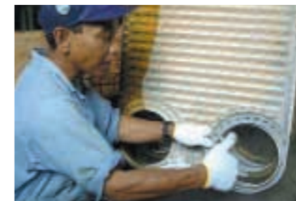
5. Plate inspection. Alfa Laval reconditioning engineers conduct another more thorough plate assessment to detect any deformation that may not have been visible with the gaskets in place.
